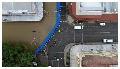
Image taken by QFES Drone capturing Fraser Coast Regional Council Levee in Maryborough. (Image courtesy of Queensland Fire and Emergency Services RPAS (Remotely Piloted Aircraft Systems) Team)
